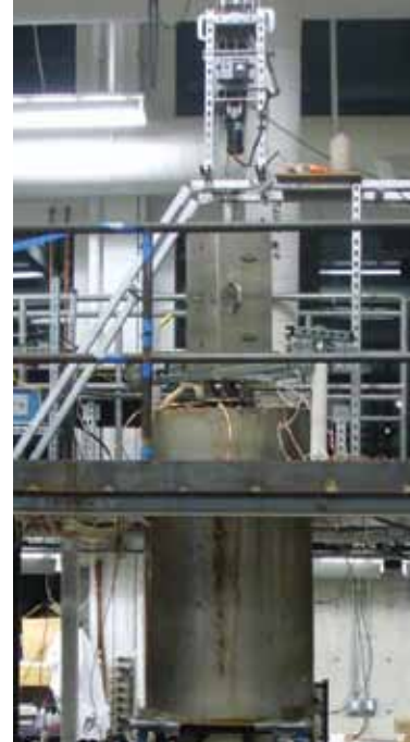
↑ FLASH SMELTER This laboratory modified reactor at the University of Utah will be replaced with a larger-scale version in 2011 that will enable longer test runs providing necessary scale-up parameters for the design and construction of an industrial pilot plant.
