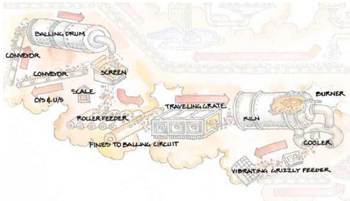
The soft pellets are then delivered to the roller feeder for final removal of the fines, which are also returned to the balling circuits. Now the soft pellets, correctly sized, are delivered to the traveling grate furnace for further drying and preheating. The grate is fired by natural gas.
