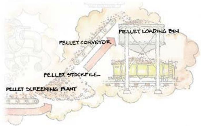
The pelletizing process has now been completed. The pellets are run through a final screening to remove those not meeting size specifications or those that are chipped or broken into fines. Pellets that meet the necessary standards are conveyed to the pellet stockpile, which holds about 30,000 tons.
