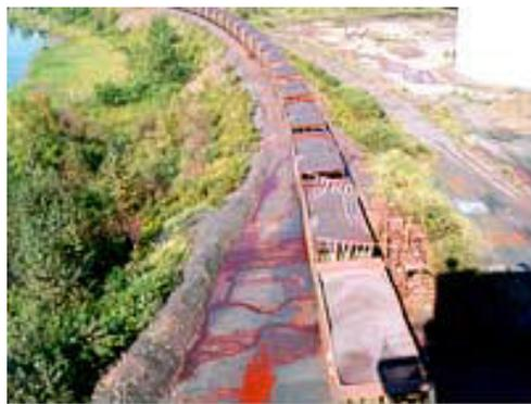
A trainload of iron ore pellets bound for the blast furnace
