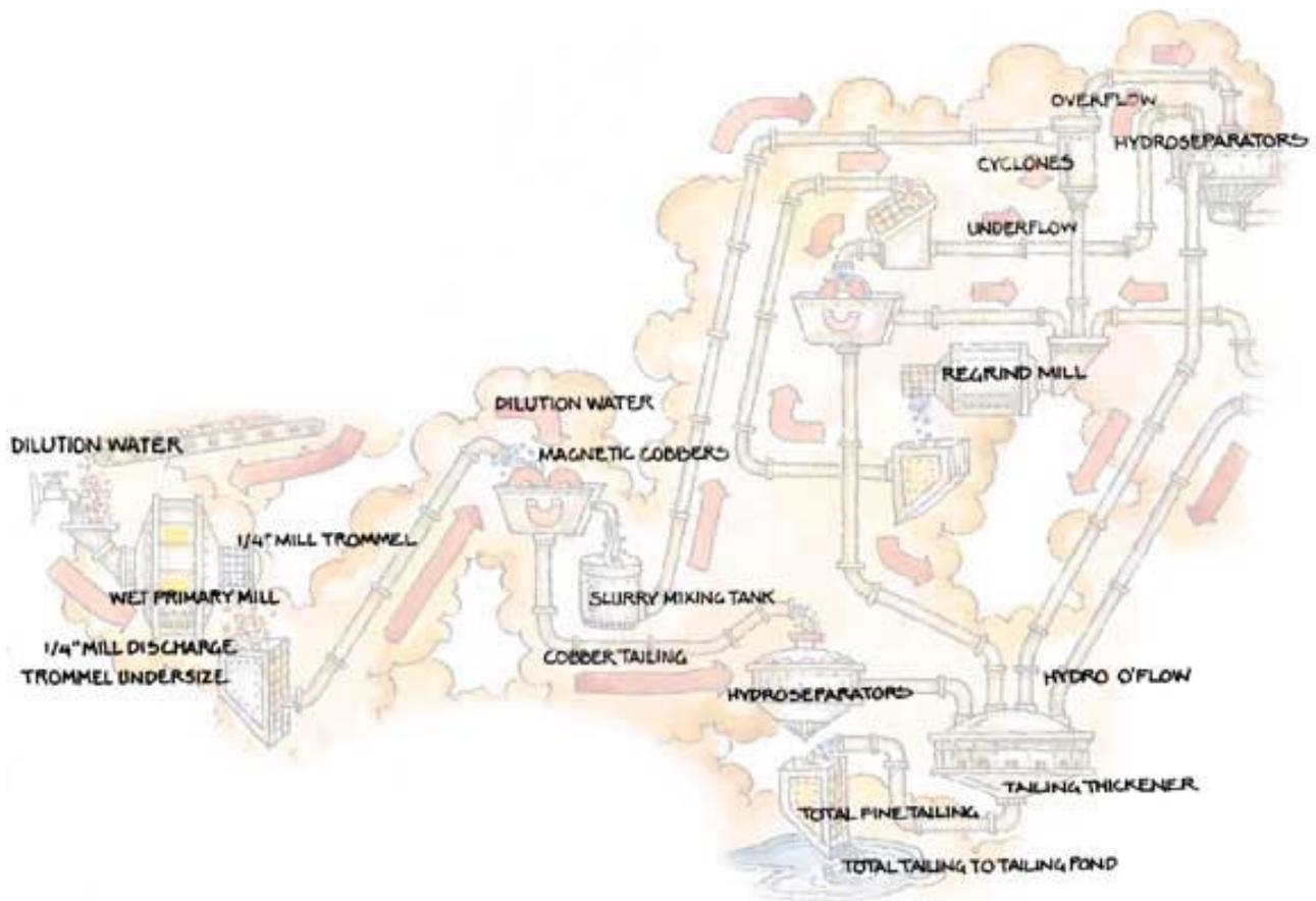
Most of the material continues to be finely ground in one of five secondary ball mills, which are powered by electric motors ranging from 2,500 hp to 4,000 hp and are charged with 1-1/2" chrome grinding balls. Fine grinding is achieved using these smaller mills, bringing the ore to a similar grind as that found in face powder. The screen undersize is then moved to hydroseparators, where silica is floated off the top.
