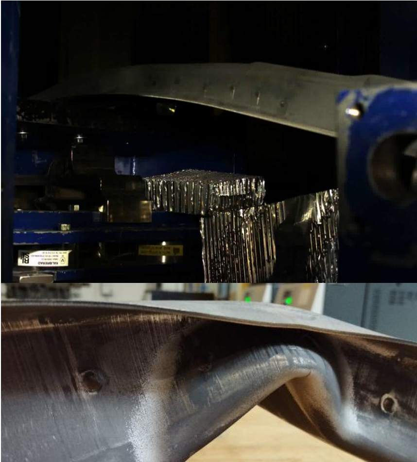
Drop Tower Test: No cracks present on the part
