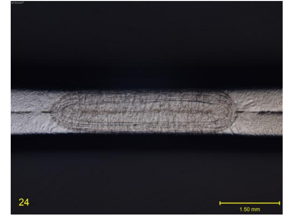
MFDC Spot Weld on a 0.8-mm to 0.8-mm 270-MPa Steel Stack-up
