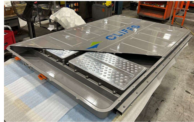
L*W*H: 2132mm*1497mm*157mm 80 kWh
