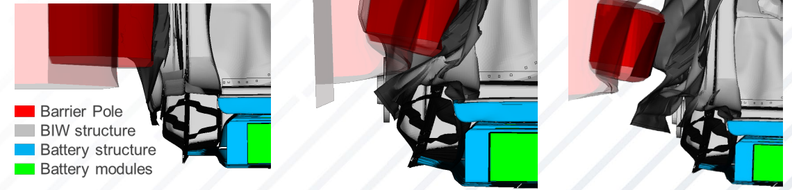
10ms Sill starts crushing 75ms midway through crush 150ms end of crush
