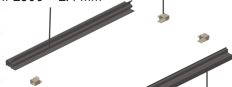
Outer-W (each side) MP1500 - 1.4 mm Frt/Rr BIW Brackets HSLA420 - 1.5 mm
