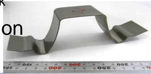
Work piece after test
