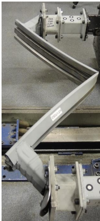
Center pole , Intrusion 460 mm AZT 16.0 km/h, 40% Offset Barrier
