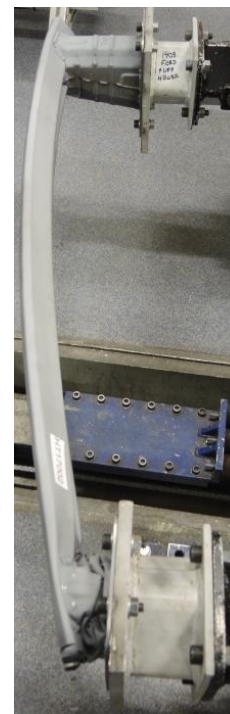
Center pole , Intrusion 460 mm AZT 16.0 km/h, 40% Offset Barrier
