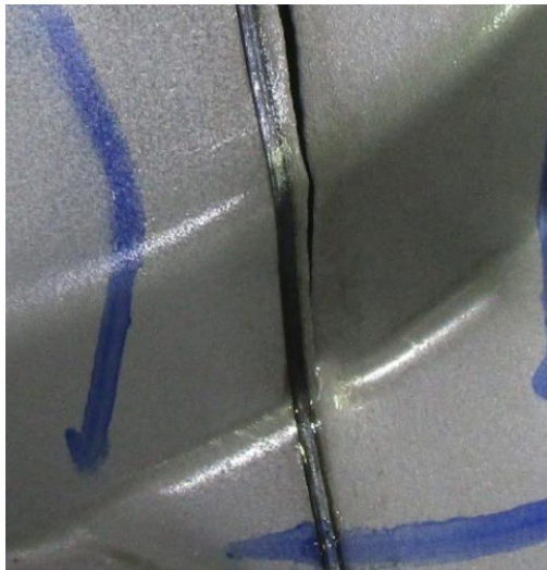
Base metal fracture
