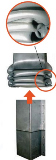
Crushing of butt-welded beams (ArcelorMittal)
