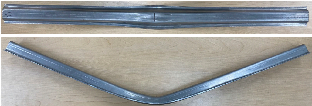
Deformed part after 6" displacement
