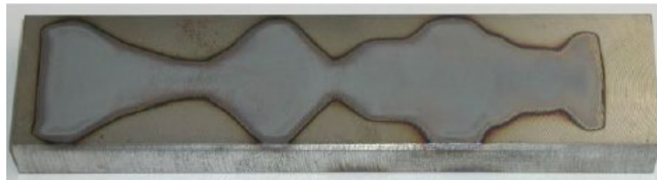
Examples of possible hardening profiles with TFC system, scanner head feed direction to left/right
