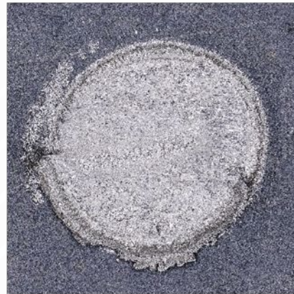
Mode 7 Interfacial Fracture
