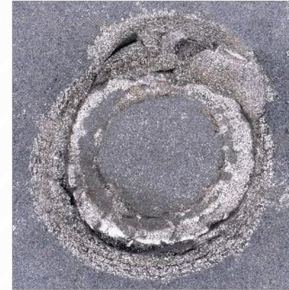
Mode 2 Partial thickness fracture with button pull
