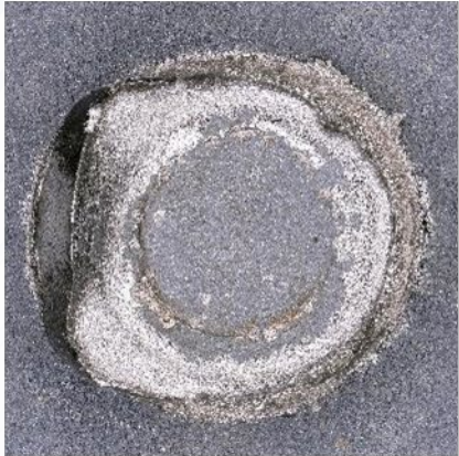
Mode 2 Partial thickness fracture with button pull
