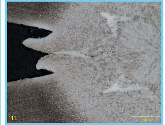
Re-filled Liquation Cracks Supplier Y Weld made with a 2-t Gap
