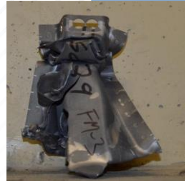
Fully martensitic Usibor® 1500-AS crush rail [2]
