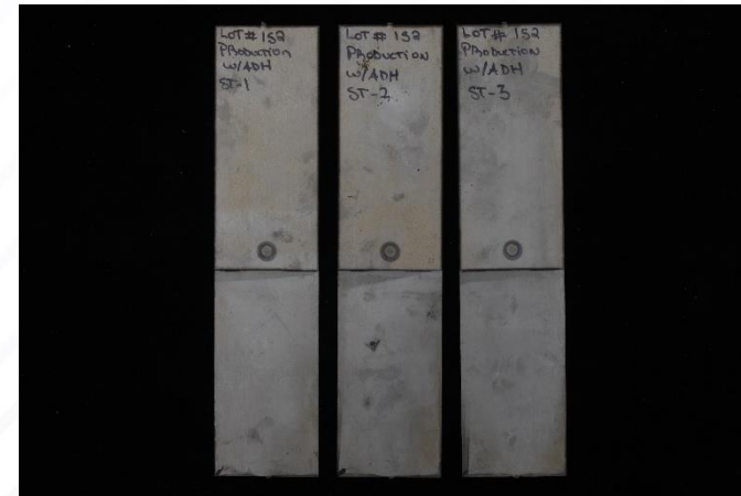
RSW (Production) with production adhesive
