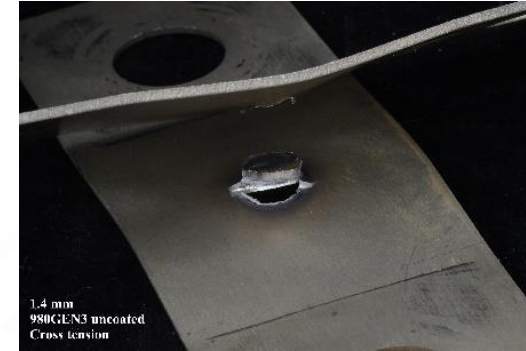
weld pullout – both sheets
