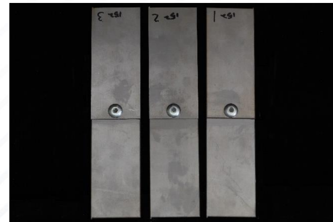
Hemlok Rivet with service adhesive
