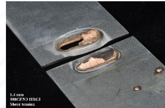
braze fracture/braze pullout – top sheet
