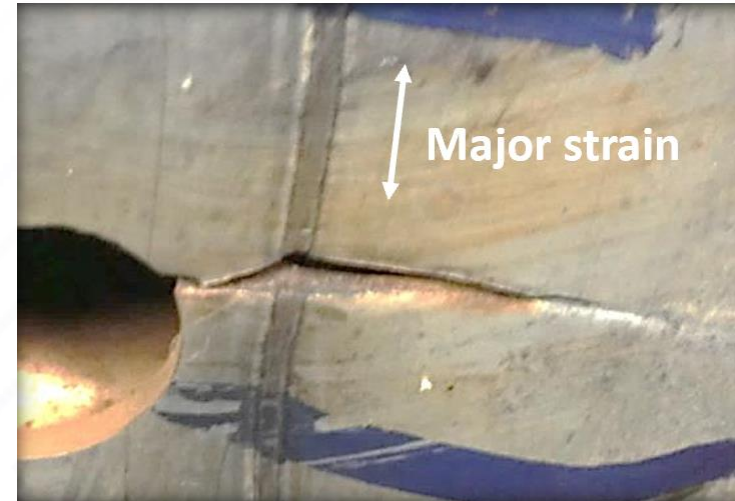
Weld fracture perpendicular to the weld seam
