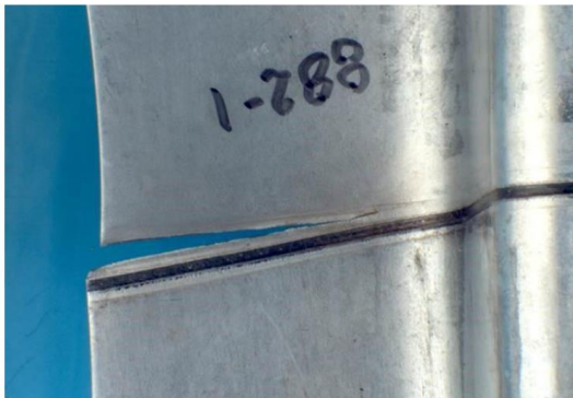
Crack/over thinning at end of weld seam
