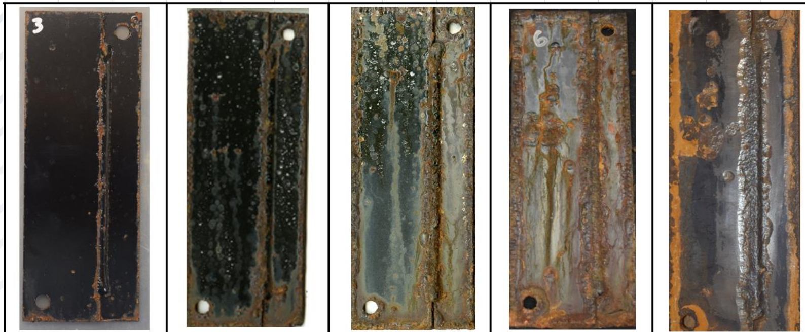
CR3 CR4 CR5 CR6 CR6 CCT 25 Cycles CCT 60 Cycles CCT 90 Cycles CCT 120 Cycles CCT 120 Cycles Rust Removed
