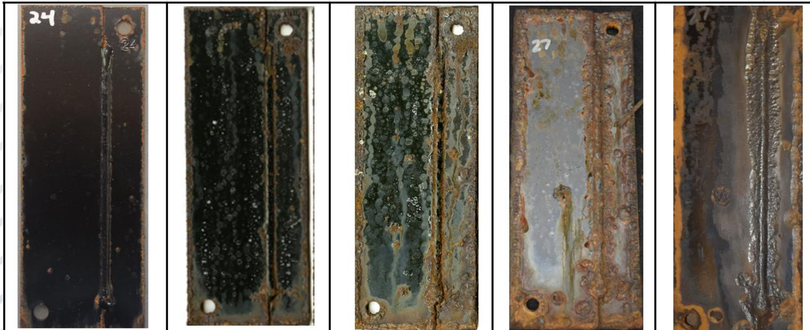
CR24 CR25 CR26 CR27 CR27 CCT 25 Cycles CCT 60 Cycles CCT 90 Cycles CCT 120 Cycles CCT 120 Cycles Rust Removed
