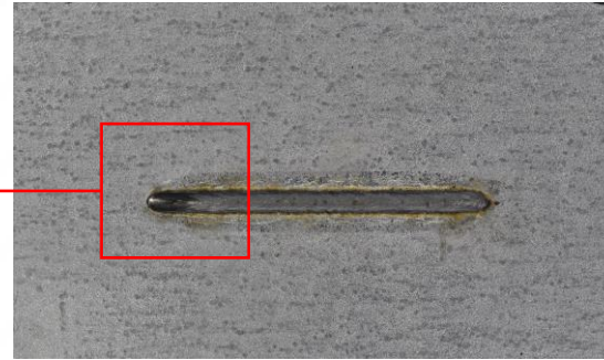
Crater crack example in Gen3 for 25mm Laser weld
