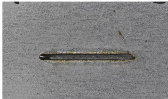
Longitudinal crack example in Gen3 for 25mm Laser weld
