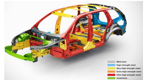
Example AHSS BIW - VOLVO XC-90 Platform
