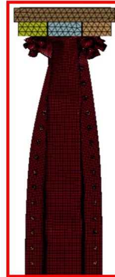
Progressive Folding (No Damage Model)
