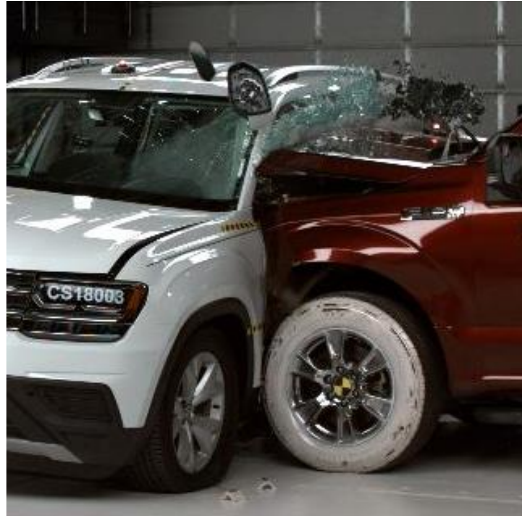
Fender and hood of F-150 crush, instead of loading a-pillar, reducing roof buckle
