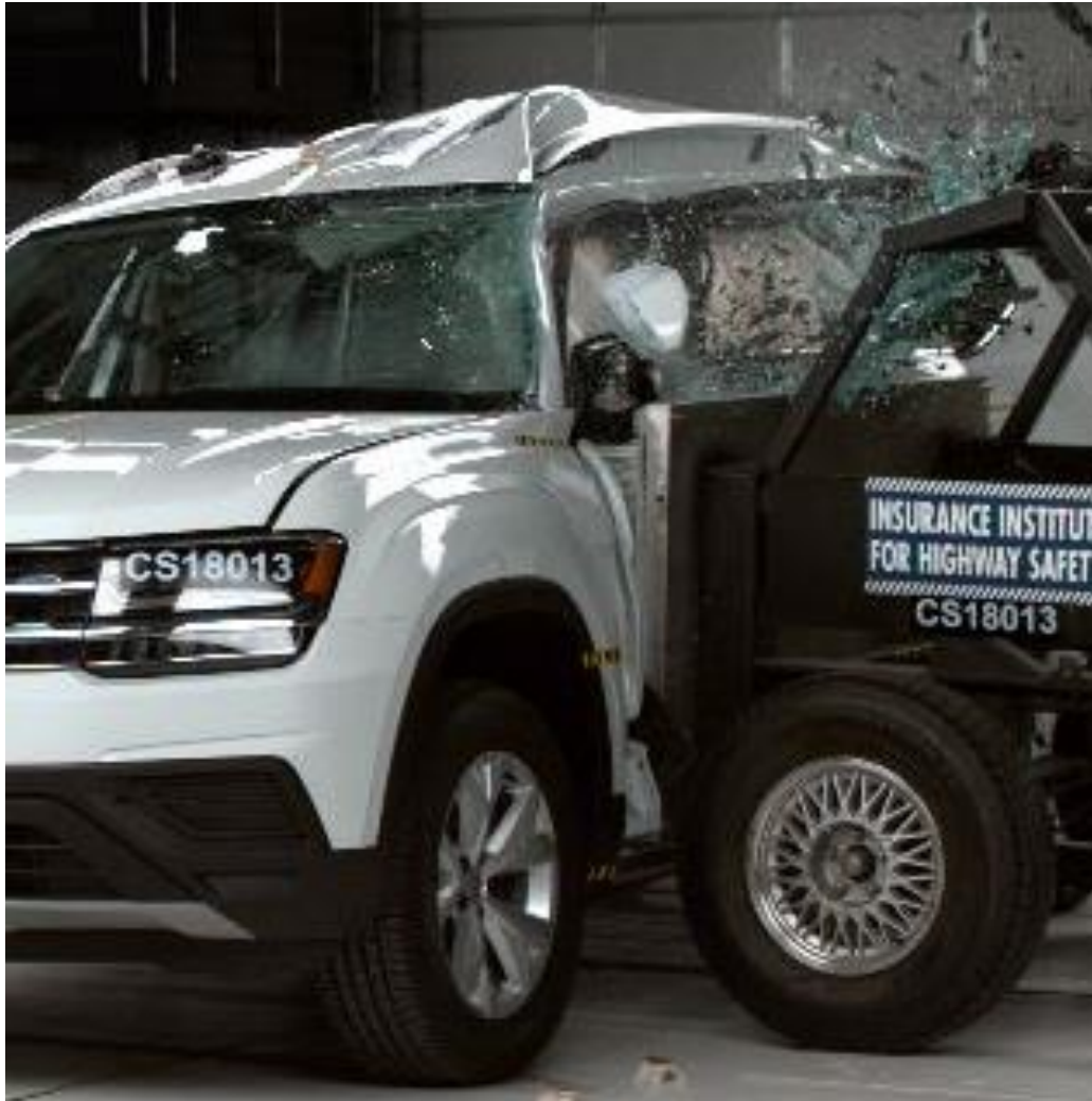
Outer edge of barrier crushes, then loads a-pillar, bucking roof and windshield
