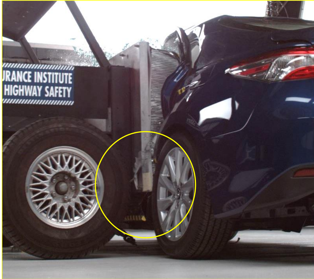
Barrier crushes and backing plate loads wheel arch
