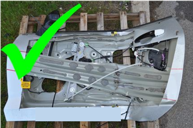
Properly processed door beam
