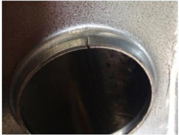
Hole Expansion (out-of-plane edge stretch)
