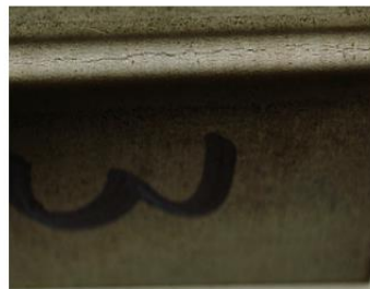
Bending Cracks over Tight Radii
