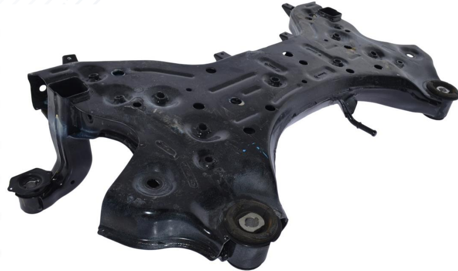
2017 Kia Sorento Small Engine Cradle Weight: 18 kg
