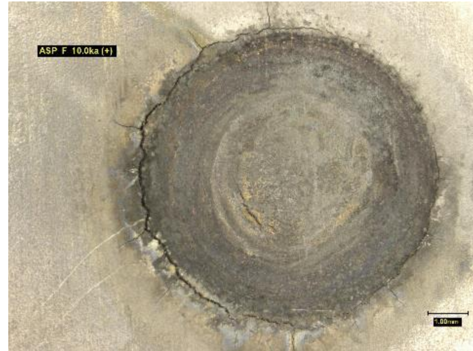
Cracks around Periphery
