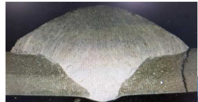
Bead-on-plate GMAW weld on a material with high LME susceptibility
