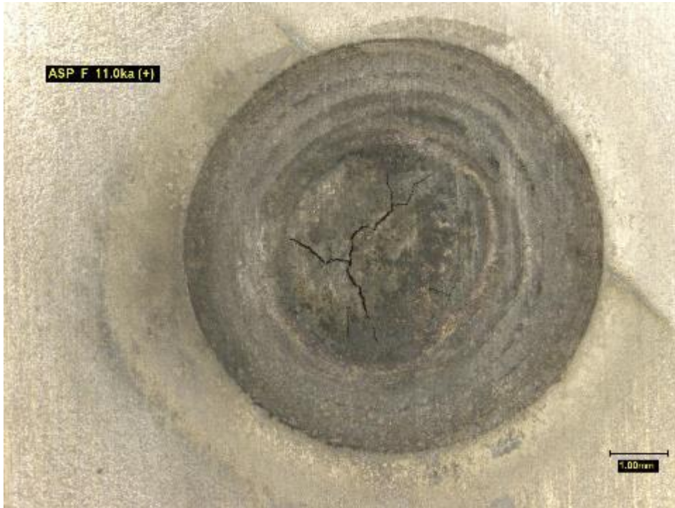
Cracks within Electrode Imprint
