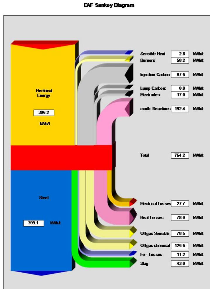
Figure 5-2. EAF Energy Input/Output (Courtesy of SMS group)
