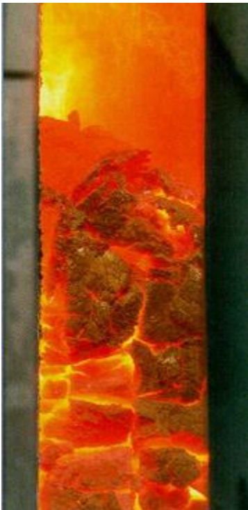
Figure 2: Incandescent coke in the oven waiting to be "pushed".
